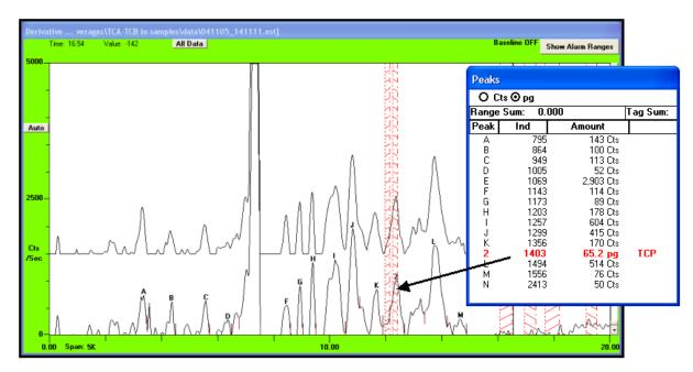
Figure 8- Two vertically offset replicate chromatograms of headspace from wood samples heated to  $40^{\circ}$ C.
