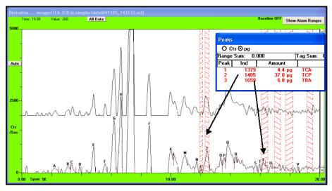
Figure 9- Headspace testing of thermally desorbed paint samples.
