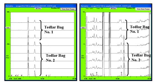
Figure 5- Replicate testing of tedlar bag air samples No. 1 & 2.
