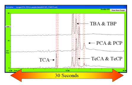
Figure 4- Vertically offset responses to anisole and phenol standards.
