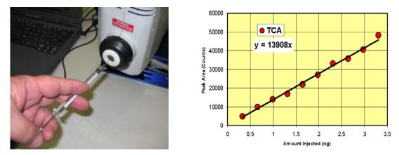
Figure 2- Direct injection of standards Figure 3- N-point calibration for TCA response
