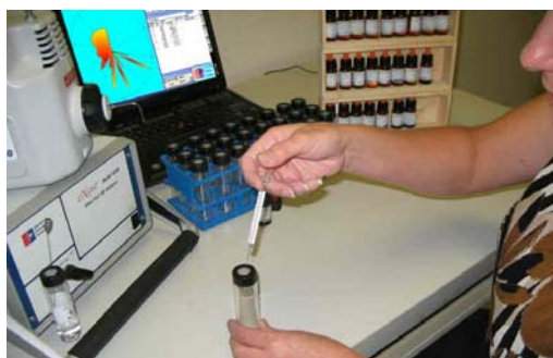
Figure 8- Step two is to inject 2 µL of fleurescence through septa and into 40 mL to create vapor sample.
