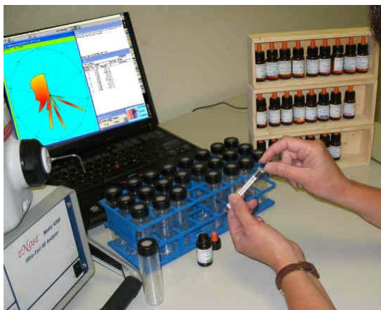
Figure 7- Step one is draw 2 µL from Fleurescence vial into a clean syringe.
