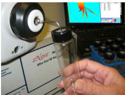
Figure 9- Step 3 is to attach vial to inlet of zNose®. A sample needle works well for volatile compounds. Above C12 compounds begin to condense onto the walls of the relatively cool sample needle.
