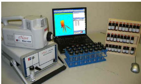
Figure 6- Testing materials are 40 mL septa sealed vials, a 1-10 µL syringe, fleurescence samples, and a zNose® vapor analyzer.
