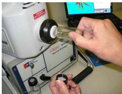
Figure 10- Removing septa cap and pressing vial against Teflon face of zNose® inlet enables direct sampling of high molecular weight compounds by the 200°C inlet of the zNose.
