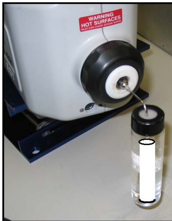
Figure 6- Direct headspace sampling of chemical odors produced from plastic samples placed in a septa-sealed vial.
