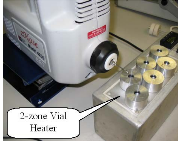
Figure 8- Direct headspace sampling of heated vials
