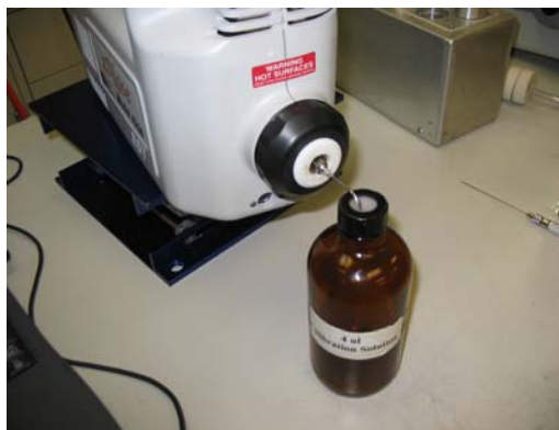
Figure 8- Direct sampling of fully vaporized gasoline samples with zNose ®
