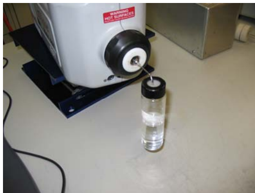
Figure 20- Direct sampling of gasoline and diesel headspace vapors with the zNose®.
